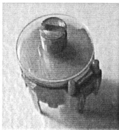
This miniature trimmer capacitor, only 7.5 mm in diameter, has a capacitance adjustable from 1.8 to 22 pF.
